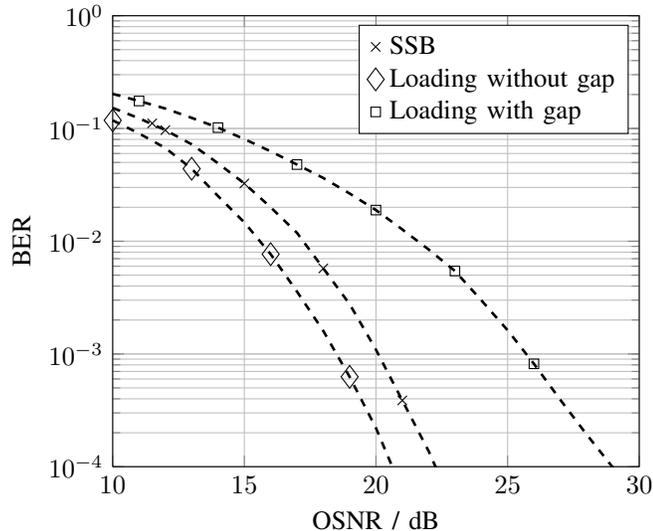
Fig. 5. Average BER with transmitter-side clipping for SSB and loading with and without gap using setup parameters as denoted in Table III with linearization of both transmitter-side and receiver-side nonlinearities
