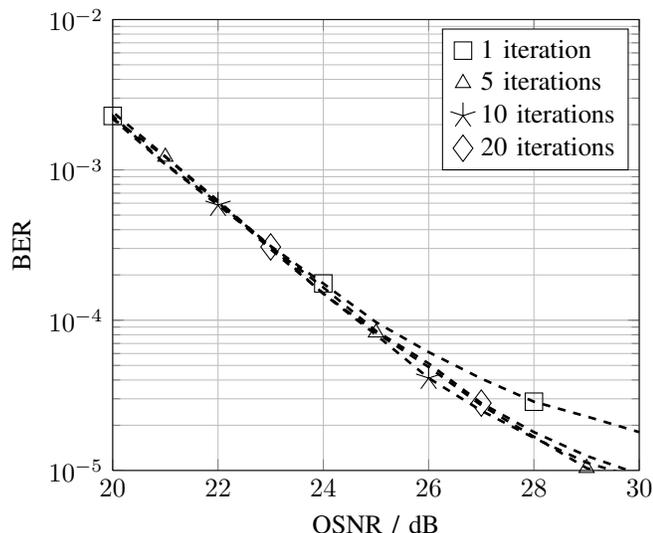
Fig. 6. Average BER loading without gap and clipping and no linearization for different number of iterations using setup parameters  $u_{\text{bias}}/V_{\pi} = -0.67$  and  $m/V_{\pi} = 0.17$
