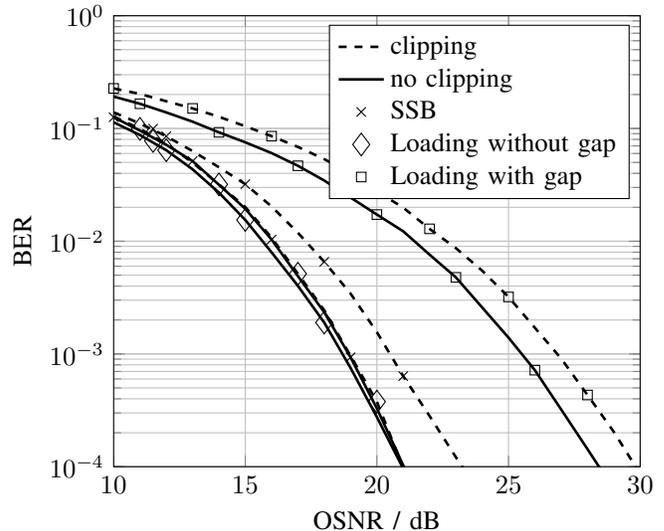
Fig. 4. Average BER with and without transmitter-side clipping for SSB and loading with and without gap using setup parameters as denoted in Table II with linearization of the receiver-side nonlinearity
