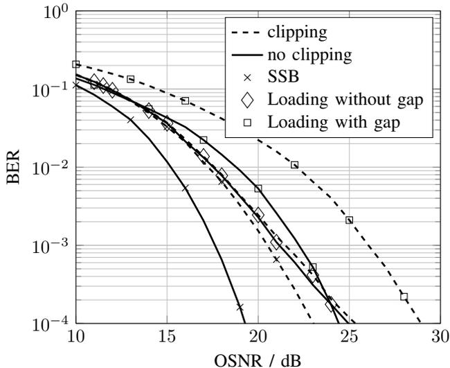
Fig. 3. Average BER with and without transmitter-side clipping for SSB and loading with and without gap using setup parameters as denoted in Table I
