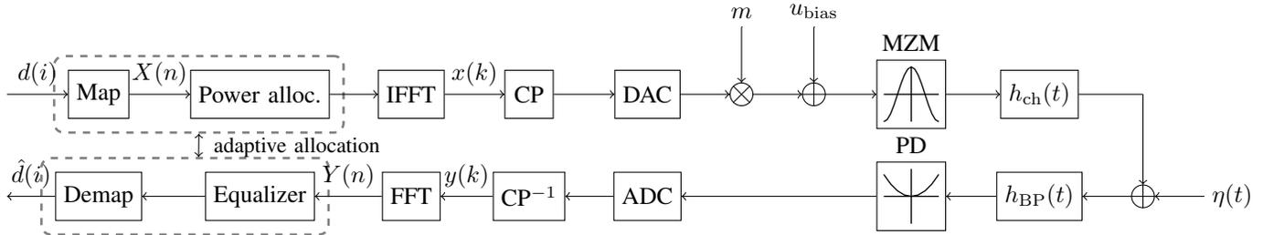
Fig. 1. Block diagram of the OFDM transmission system with bit and power loading
