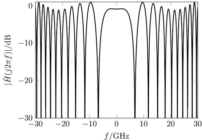
Fig. 2. Frequency response of the equivalent channel for a fiber length of 80 km and a dispersion constant of 17 ps/(nm·km)
