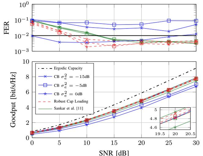
Fig. 4. Goodput and FER vs. SNR with genie code rate and a design gap  $\epsilon_{R_C} = 0.07$ ; OFDM parameters:  $N_C = 1024$ ,  $L = 10$  equal power Rayleigh fading taps.
