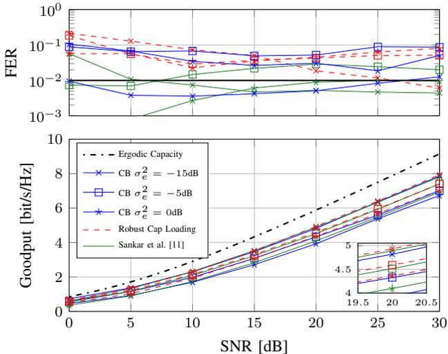
Fig. 5. Goodput and FER vs. SNR for robust and non-robust bit and power loading with LTE turbo code fitted to estimated  $\hat{R}_C$ ,  $\epsilon_{R_C} = \{0.06, 0.04, 0\}$  variable, but fixed  $\epsilon_{R_C} = 0.07$  for Sankar et al.; OFDM parameters:  $N_C = 1024$ ,  $L = 10$  equal power Rayleigh fading taps.
