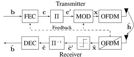
Fig. 1. Adaptive OFDM System Model.
