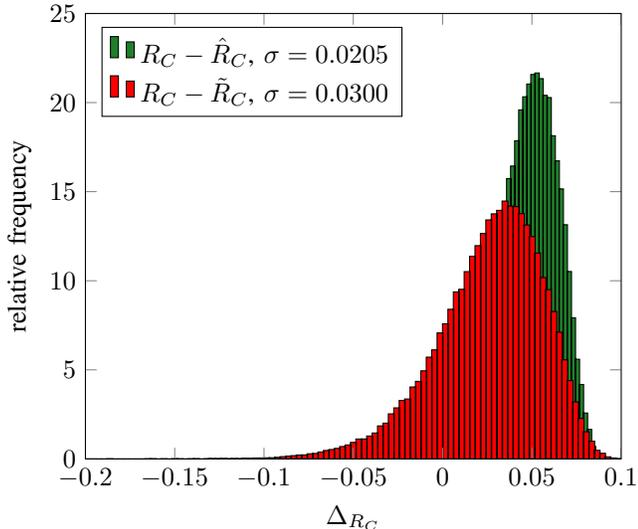
Fig. 3. Histograms of the errors in code rate estimation  $R_C - \hat{R}_C$  and  $R_C - \tilde{R}_C$  using robust bit and power loading; SNR = 20dB,  $\delta = 0.01$ ,  $N_C = 1024$ ,  $L = 10$  equal power Rayleigh fading taps.
