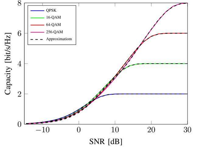
Fig. 2. Comparison of approximated capacity and true capacity for various modulations
