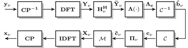
Fig. 1. Structure of the  $\nu$ -th OFDM-IDM-STC-relay.
