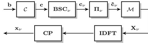
Fig. 2. Equivalent model for the transmitter and the  $\nu$ -th relay based on a binary symmetric channel describing the correlation between the transmitter's codeword  $c$  and the relay's codeword  $c_\nu$ .
