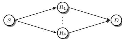
Fig. 3. Topology of the considered two-hop relay-system with one source  $S$ , one destination  $D$  and  $N = 4$  parallel relays  $R_\nu$ .
