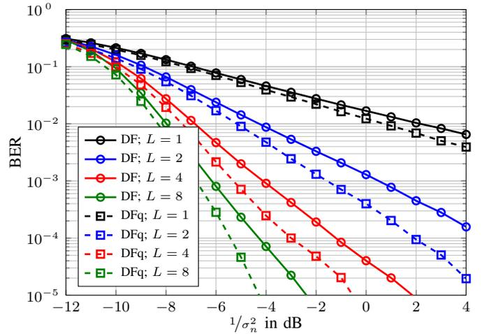
Fig. 5. Comparison of the achieved bit-error-rates with (DFq) and without (DF) considering the relay's error probabilities in the decoding process at the destination for a varying number of channel taps  $L$ .  $N = 4$  relays.  $(5; 7)_8$ -convolutional code and half-rate repetition code. Frame length  $L_{f,c} = 1024$  codebits. QPSK signaling. Soft-rake-detection with  $N_{it} = 10$  iterations.  $N_c = 64$  subcarriers. Length of cyclic prefix  $L_{CP} = 8$ .
