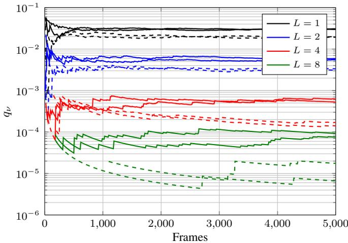
Fig. 4. Long-term statistics of the error probabilities  $q_\nu$  at the relays versus the number of transmitted frames for a varying number of channel taps  $L$  at  $1/\sigma_n^2 = 0$  dB. Solid: outer relays, dashed: inner relays.
