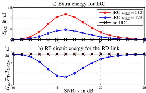
Fig. 4. a) Extra total energy consumption for IRC  $\mathcal{E}_{\text{IRC}}$ . b) RF circuit energy consumption for the RD link  $K_{\text{act}} \mathcal{E}_{\text{Tx}}$ .
