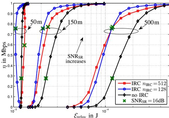
Fig. 5. Energy at relays versus throughput during one transmission from S to D for different distances and different number of exchanged bits in IRC.
