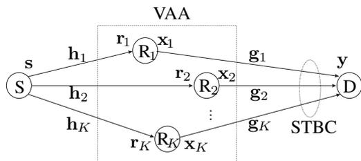
Fig. 1. Distributed relaying system with  $K$  relays constituting a VAA. In case of no IRC, all relays participate in the transmission to D using STBC.
