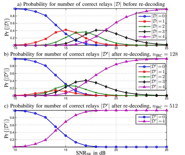
Fig. 3. Probability distributions for the number of correct relays a) before and b), c) after re-decoding with  $n_{\text{IRC}} = 128, 512$  punctured bits exchange.
