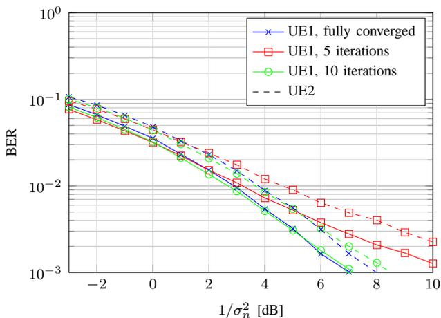
Fig. 5. Simulated bit error rates for a system in line topology with 2 UEs transmitting 2 spatial layers each, and 3 receiving iSCs with 4 antennas each using the distributed estimation algorithm for a fixed number of iterations (5 and 10) and iteration until convergence is achieved
