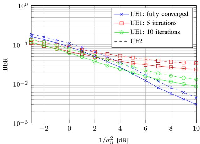
Fig. 4. Simulated bit error rates for a system in ring topology with 2 UEs transmitting 4 spatial layers each, and 3 receiving iSCs with 4 antennas each using the distributed estimation algorithm for a fixed number of iterations (5 and 10) and iteration until convergence is achieved
