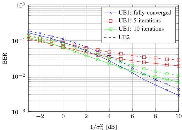
Fig. 6. Simulated bit error rates for a system in line topology with 2 UEs transmitting 4 spatial layers each, and 3 receiving iSCs with 4 antennas each using the distributed estimation algorithm for a fixed number of iterations (5 and 10) and iteration until convergence is achieved
