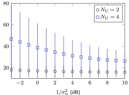
Fig. 3. Average number of required iterations  $\pm$  standard deviation for convergence in the case of a ring topology
