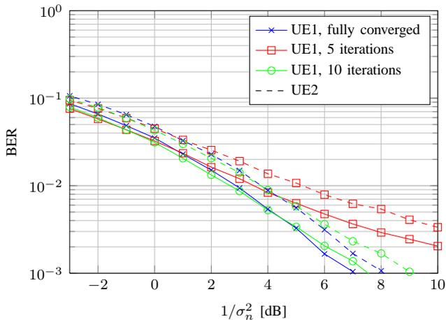
Fig. 2. Simulated bit error rates for a system in ring topology with 2 UEs transmitting 2 spatial layers each, and 3 receiving iSCs with 4 antennas each using the distributed estimation algorithm for a fixed number of iterations (5 and 10) and iteration until convergence is achieved
