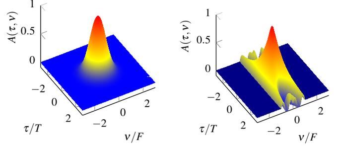
(a) Gaussian prototype filter (b) Rectangular prototype filter
