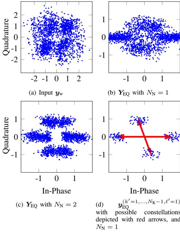
Fig. 6. Equalizer signals of a whole frame. (a) equalizer input given by (7), (b) and (c) equalizer output in (17), and (d) output signal at one specific time instance
