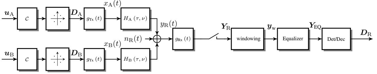
Fig. 2. Block diagram of the MA phase of a PLNC system with Generalized FDM (GFDM)
