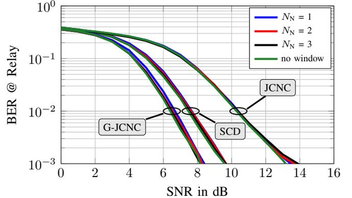
Fig. 7. BER performance at the relay of SCD, JCNC and G-JCNC using Gaussian transmit and receive filter, including the effect of delay and Doppler.  $\tau_i < \tau_{\max} = 0.08T$ ,  $|\nu_i| < \nu_{\max} = 0.08F$ .
