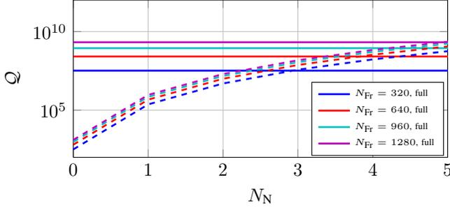
Fig. 5. Complexity of a full inversion (—), and inversion of reduced size matrix (- -)
