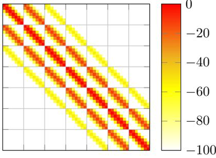
Fig. 4. Absolute values of the elements in matrix  $\mathbf{V}_i$  for one user in logarithmic scale
