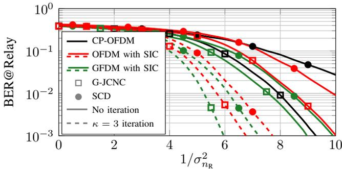
Fig. 5. Impact of BER performance with additional CFOs  $\Delta\nu^{(A)} = 0.1F$  and  $\Delta\nu^{(B)} = -0.1F$  and G-JCNC and SCD,  $\tau_{\max} = 0.2T$  and  $\nu_{\max} = 0$
