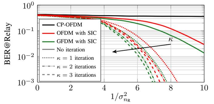
Fig. 6. Iterations analysis in channels with high additional CFOs of  $\Delta\nu_A = 0.2F$  and  $\Delta\nu_B = -0.2F$ .  $\tau_{\max} = 0.2T$  and  $\nu_{\max} = 0$
