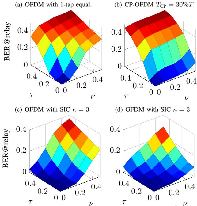
Fig. 8. BER performance at the relay with noise variance  $1/\sigma_{n_R}^2 = 5\text{dB}$  with different  $\tau_{\max}$  and  $\nu_{\max}$ .
