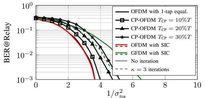
Fig. 3. Frequency flat channel, no delay spread  $\tau_{\max} = 0$ , no Doppler spread  $\nu_{\max} = 0$ ,  $\Delta\nu_A = 0$  and  $\Delta\nu_B = 0$ , PLNC detection scheme: G-JCNC
