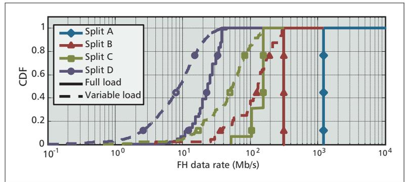
**Figure 3.** Cumulative distribution function (CDF) of required FH data rates of different functional splits considering full load in all BSs (solid lines) and considering a varying load (dashed lines).
