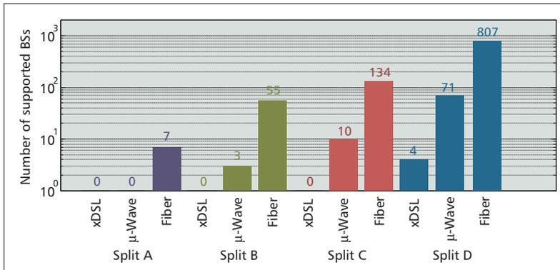
**Figure 5.** Number of BSs supported by different FH technologies: xDSL@100 Mb/s,  $\mu$ -Wave@1 Gb/s, fiber@10 Gb/s.
