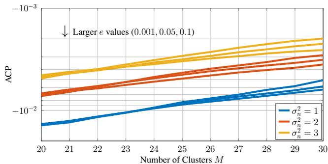
Fig. 4. ACP vs. number of clusters  $M$ , 16-QAM signaling, AWGN access channel with  $\sigma_n^2 = 1, 2, 3$ , forward channel with  $\epsilon = 0.1, 0.05, 0.001$
