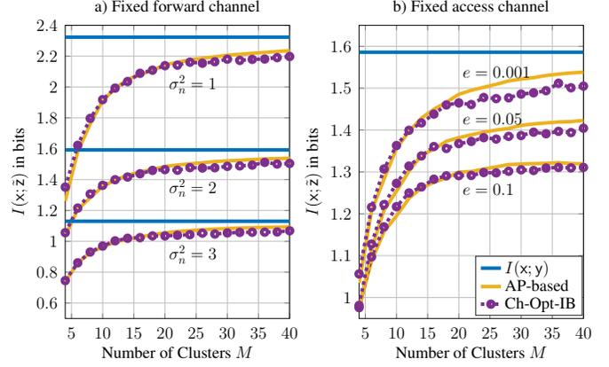
Fig. 3. Overall transmission rate  $I(x; \tilde{z})$  vs. number of clusters  $M$ , 16-QAM signaling: a) fixed forward channel with reliability  $e = 0.001$ , AWGN access channel with  $\sigma_n^2 = 1, 2, 3$  and b) fixed AWGN access channel with  $\sigma_n^2 = 2$ , forward channel with reliabilities  $e = 0.1, 0.05, 0.001$
