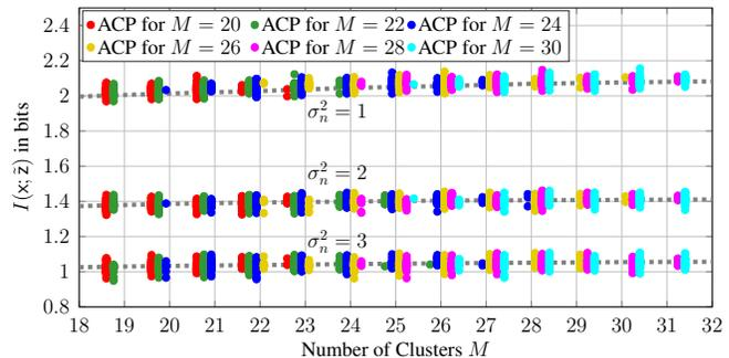
Fig. 5. Overall transmission rate  $I(x; \bar{z})$  vs. number of clusters  $M$ , 16-QAM signaling, AWGN access channel with  $\sigma_n^2 = 1, 2, 3$ , forward channel with  $e = 0.05$ , bisection result (---), slight misalignment for overlap prevention
