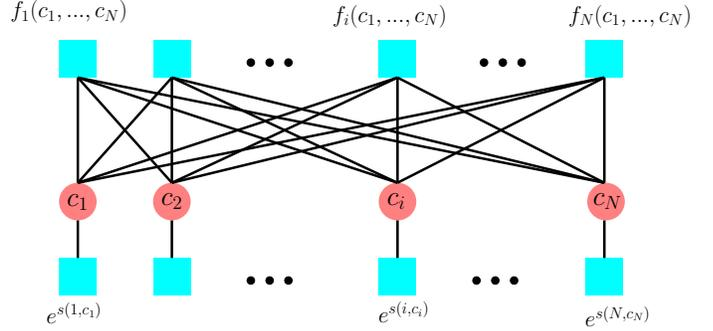
Fig. 2. The factor graph on which AP is developed, the *factor nodes*  $f_i$  and the *variable nodes*  $c_i$  with  $i \in \{1, \dots, N\}$  represent the *coherency check* and the *chosen exemplar* for the article  $i$ , respectively
