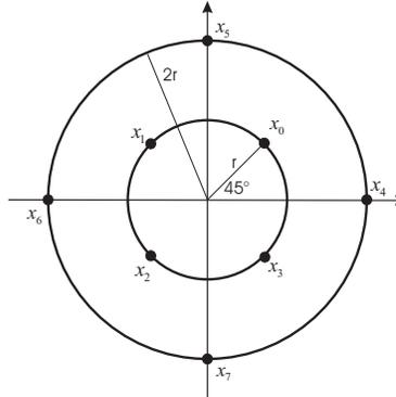
**Fig. 1:** Field of signals for the 8-ASK/PSK constellation
