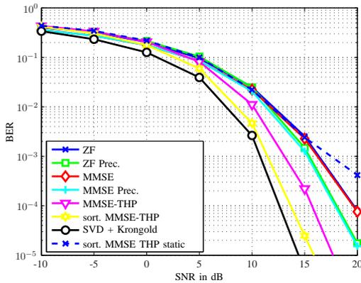
Fig. 4. a) Mean BER of different transmission schemes for  $N_R = N_T = 4$  antennas at 16 bit/s/Hz;  $N_C = 1024$  subcarriers,  $N_U = 5$  users and  $L_F = 6$ .
