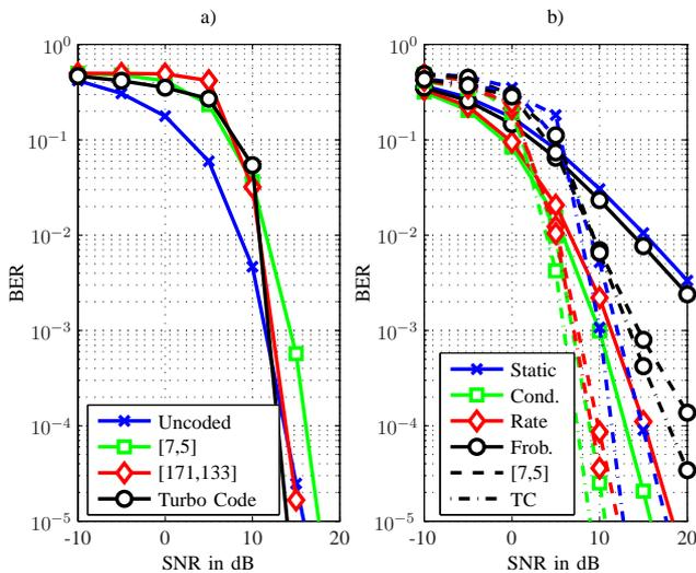
Fig. 6. Mean BER of a) sorted MMSE THP coded with different codes for  $N_R = N_T = 4$  antennas and 16 bit/s/Hz and b) Spatial multiplexing for  $N_R = N_T = 4$  with different codes at 8 bit/s/Hz;  $N_C = 1024$  subcarriers,  $N_U = 5$  users,  $L_F = 6$  and rate metric.
