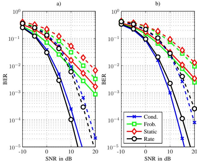
Fig. 3. a) Spatial multiplexing with receiver side ZF filtering and  $N_R = N_T = 2$  antennas (— 4 bit/s/Hz, --- 8 bit/s/Hz), b)  $N_R = N_T = 4$  antennas (— 8 bit/s/Hz, --- 16 bit/s/Hz);  $N_C = 1024$  subcarriers,  $N_U = 5$  users and  $L_F = 6$ .
