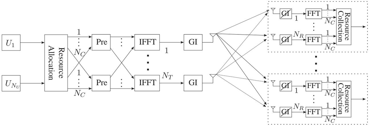
Fig. 1. System model with transmitter side precoding
