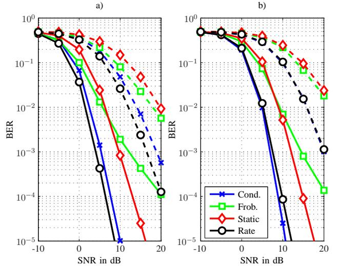
Fig. 5. a) Mean BER for a [7, 5] coded spatial multiplexing system with receiver side ZF filtering at  $N_R = N_T = 2$  antennas (— 4 bit/s/Hz, --- 8 bit/s/Hz), b)  $N_R = N_T = 4$  antennas (— 8 bit/s/Hz, --- 16 bit/s/Hz);  $N_C = 1024$  subcarriers,  $N_U = 5$  users and  $L_F = 6$ .
