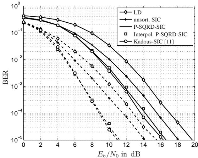
**Fig. 6.** BER of LD and SIC with respect to the ZF (–) or the MMSE (– –) criterion for a PAC MIMO-OFDM system with  $N_T = N_R = 4$  antennas, channel order  $N_H = 5$ ,  $N_C = 128$  subcarriers, guard interval of length  $N_G = 5$ , 4-QAM
