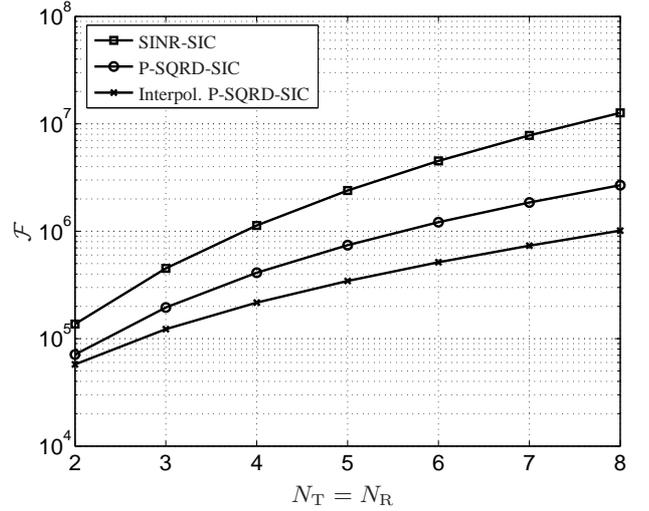
**Fig. 5.** Number of floating point operations  $\mathcal{F}$  for SINR-SIC, P-SQRD-SIC and interpolated P-SQRD-SIC detection with respect to the ZF criterion of a MIMO-OFDM system with  $N_T = N_R$  antennas,  $N_C = 1024$  subcarriers and channel order  $N_H = 8$
