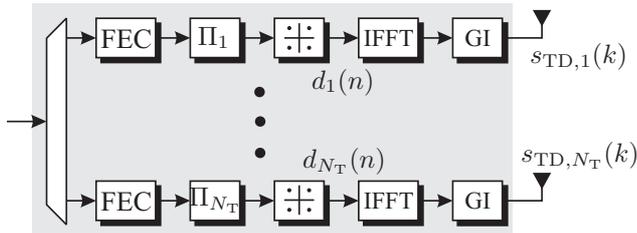
Fig. 1. MIMO-OFDM transmitter with per-antenna coding
