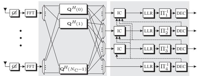
**Fig. 2.** Successive interference cancellation for a MIMO-OFDM scheme with  $N_T = 4$  transmit antennas
