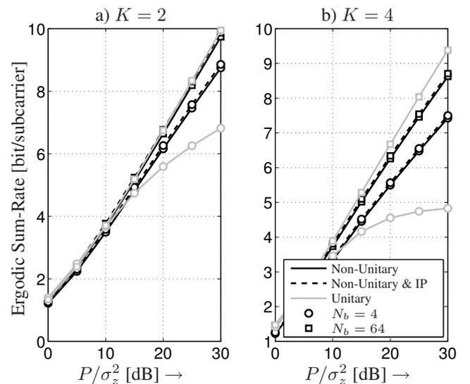
**Fig. 4.** Average ergodic sum-rate vs. SNR for different BF schemes and codebook sizes  $N_b$  for a chunk size of  $N_f \times N_s = 16 \times 6$
