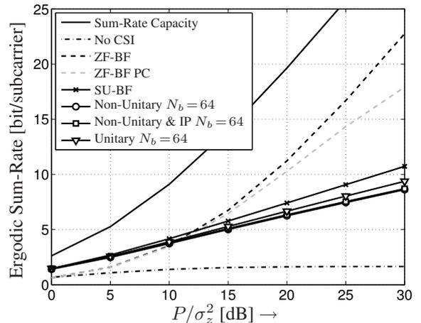
**Fig. 6.** Average ergodic sum-rate vs. SNR for different schemes with  $K = 4$  users and a chunk size of  $N_f \times N_s = 16 \times 6$
