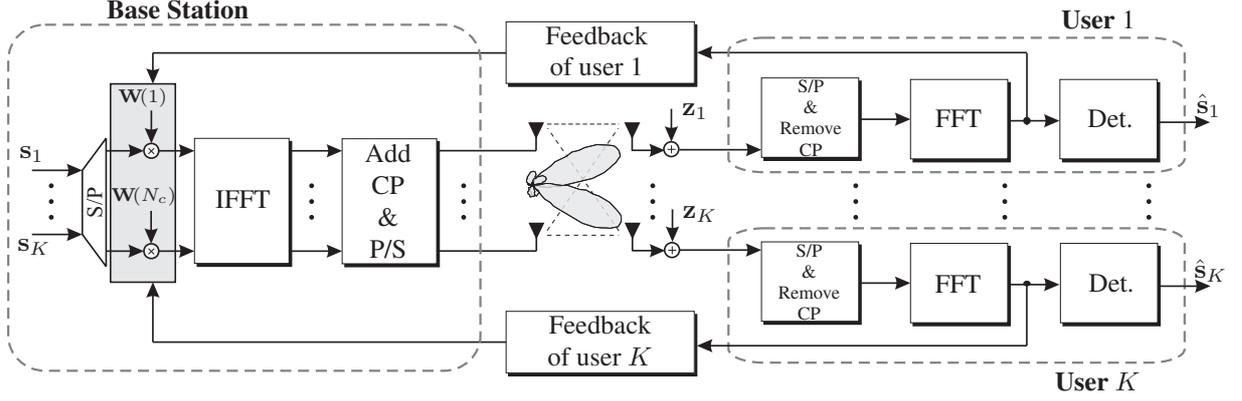
**Fig. 1.** Block diagram of a multi-user MISO-OFDM system with  $N_T$  transmit antennas,  $K$  users and  $N_c$  sub-carriers with linear precoding
