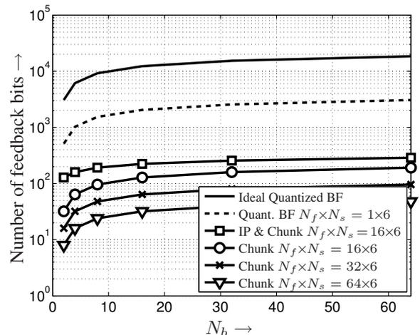
**Fig. 3.** Number of feedback bits vs. codebook size for the compared schemes with  $N_c = 512$  and  $R = 8$
