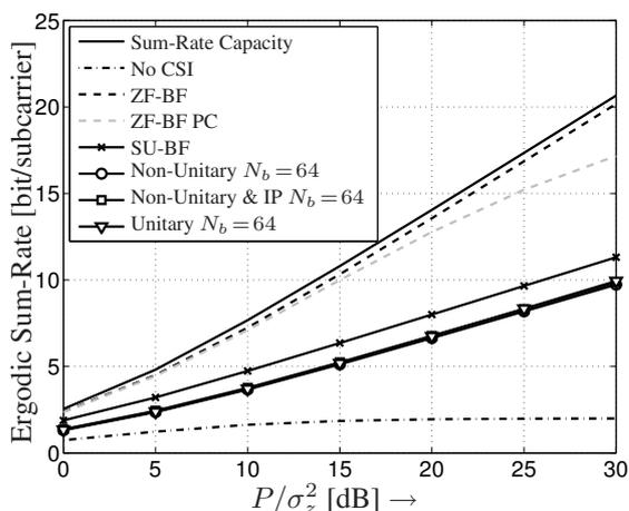
**Fig. 5.** Average ergodic sum-rate vs. SNR for different schemes with  $K = 2$  users and a chunk size of  $N_f \times N_s = 16 \times 6$
