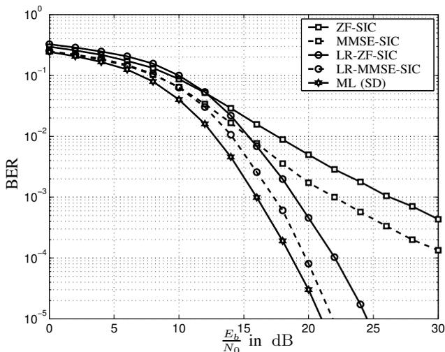
Fig. 10. Bit Error Rate of a system with  $n_T = 4$  and  $n_R = 4$  antennas, 16-QAM symbols, ZF (continuous lines) and MMSE (dashed lines) optimally sorted SIC detection.
