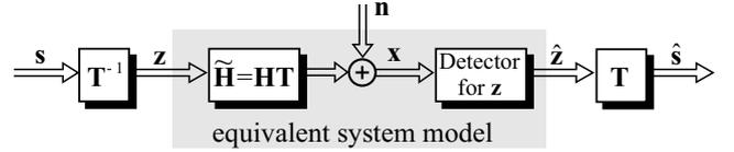
Fig. 4. Block diagram of a Lattice-Reduction based detector.
