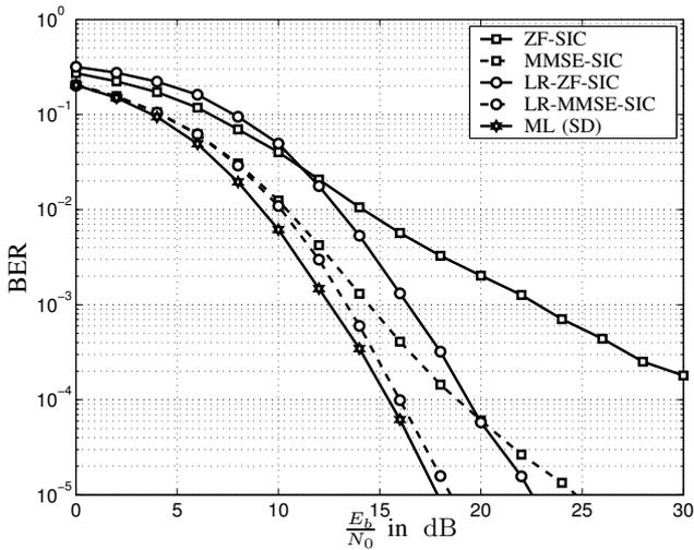
Fig. 13. Bit Error Rate of a system with  $n_T = 4$  and  $n_R = 4$  antennas, 4-QAM symbols, ZF (continuous lines) and MMSE (dashed lines) optimally sorted SIC detection with imperfect CSI due to channel estimation with  $L = 12$  pilot symbols.
