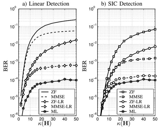
Fig. 9. Bit Error Rates versus condition number  $\kappa(\mathbf{H})$  for a system with  $n_T = 4$  and  $n_R = 4$  antennas, 4-QAM symbols,  $E_b/N_0 = 16$  dB, ZF (continuous lines) and MMSE (dashed lines) a) linear detection and b) SIC detection.
