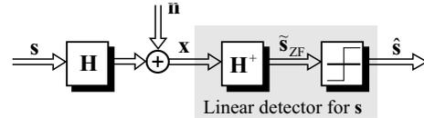
Fig. 2. Block diagram of linear zero-forcing detection.
