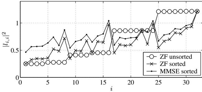
Fig. 3. Influence of sorting and MMSE filtering on  $|l_{i,i}|^2$
