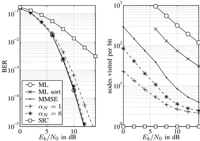
Fig. 6. Bit error rates and complexity of detection algorithms ( $\alpha_1 = 8$ ).
