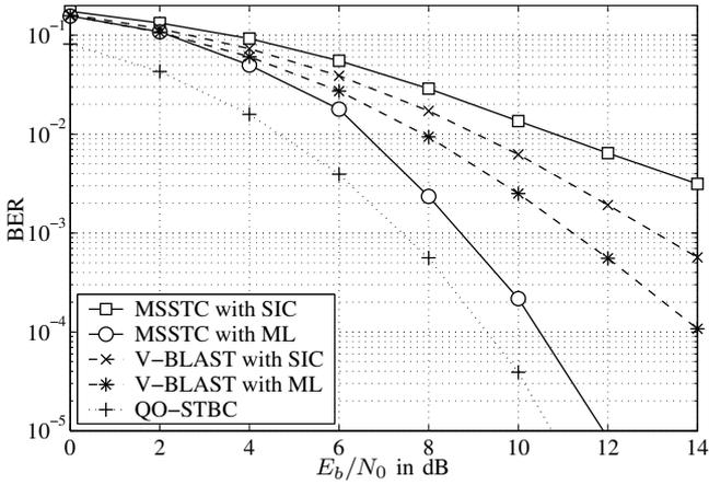
Fig. 5. Bit error rates for MSSTC and V-BLAST with SIC and ML detection. The quasi-orthogonal space-time block code from (9) serves as reference.
