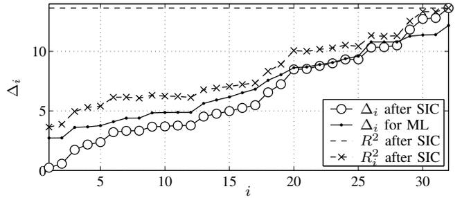
Fig. 4. Cumulative Distances  $\Delta_i$  after initial SIC and for ML solution. Also shown are the initial squared radii  $R^2$  and  $R_i^2$  for  $\alpha_1 = 8$  and  $\alpha_N = 1$ .
