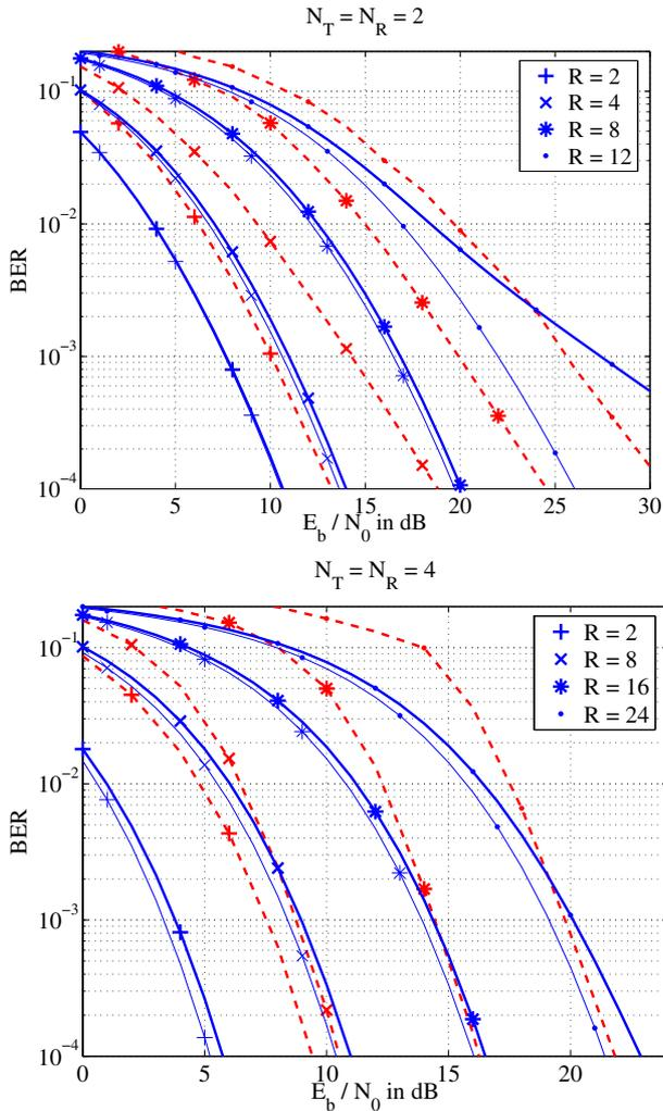
**Fig. 2.** Bit error rates for multistratum space-time codes (dashed) and adaptive transmission with  $R_i \in \{2, 4, 6, 8\}$  (solid). The thin lines correspond to waterfilling without discrete rate constraints.
