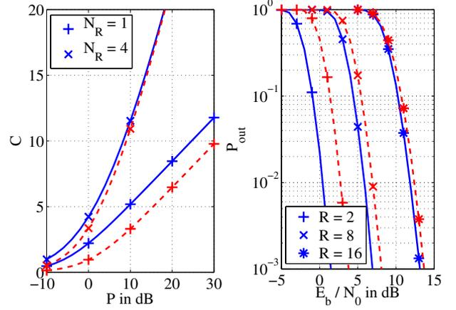
**Fig. 1.** Ergodic channel capacity for  $N_T = 4$  (left) and outage probability for  $N_T = N_R = 4$  (right) with waterfilling (solid) and equal power allocation (dashed).
