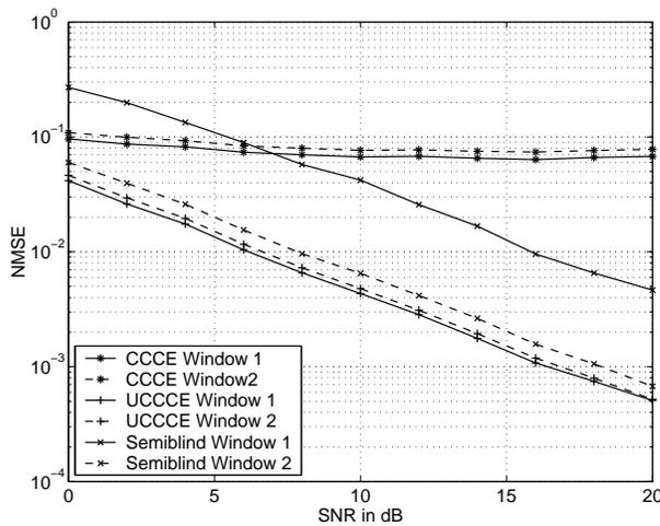
**Figure 2:** NMSE vs. SNR for a CDMA system with 1 active user
