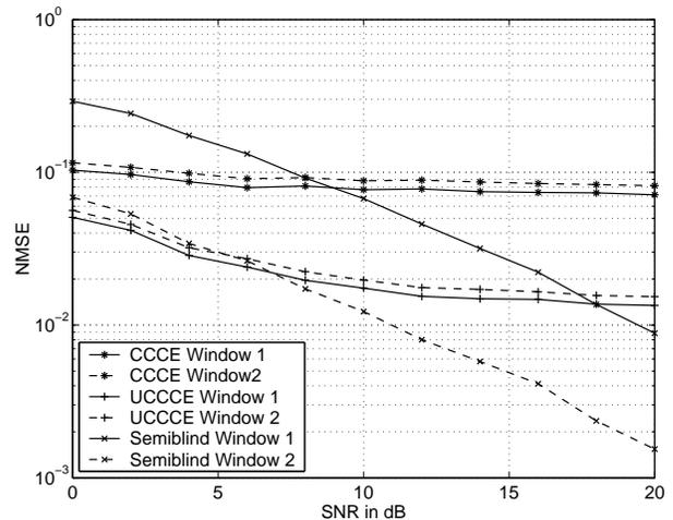
**Figure 3:** NMSE vs. SNR for a CDMA system with 15 active users and one pilot channel
