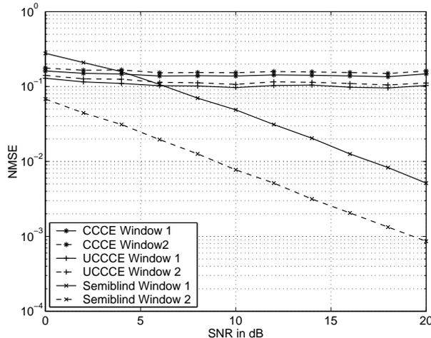
**Figure 4:** NMSE vs. SNR for a CDMA system under extreme near-far conditions with 6 active user
