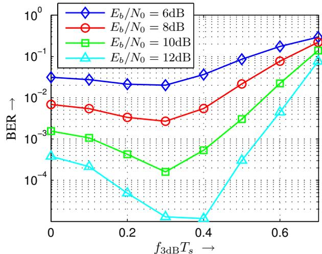
Fig. 3. Performance comparison of different  $f_{3\text{dB}}$ -bandwidths for the multicarrier system with truncated Gaussian impulses
