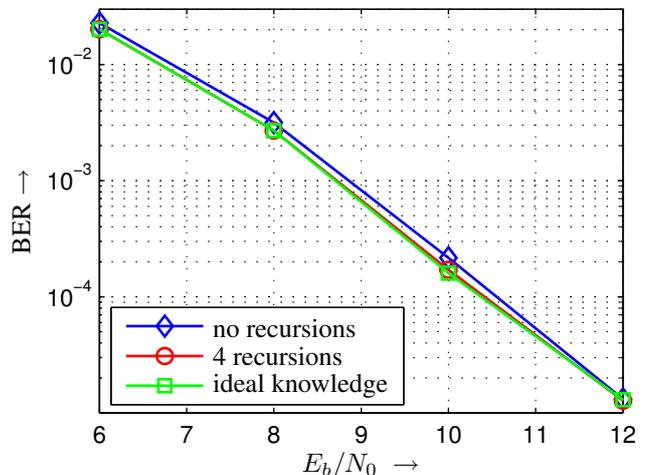
Fig. 5. Bit error rates for the tailbiting Max-Log-MAP equalization with ideal knowledge of the first and last channel state, with no recursions, and with 4 recursions
