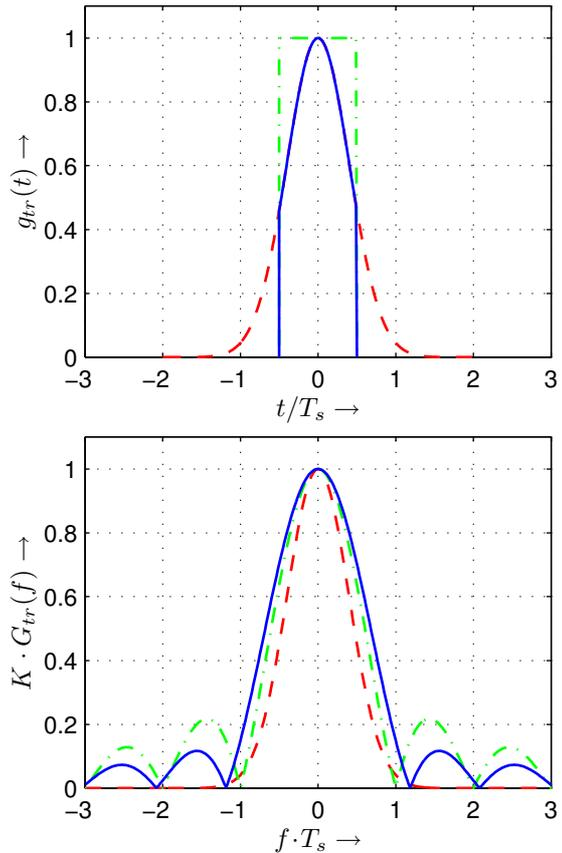
Fig. 1. Normalized Gaussian (— —), rectangular (— · —), and truncated Gaussian impulse (—) in time and frequency domain with  $f_{3\text{dB}} T_s = 0.3$
