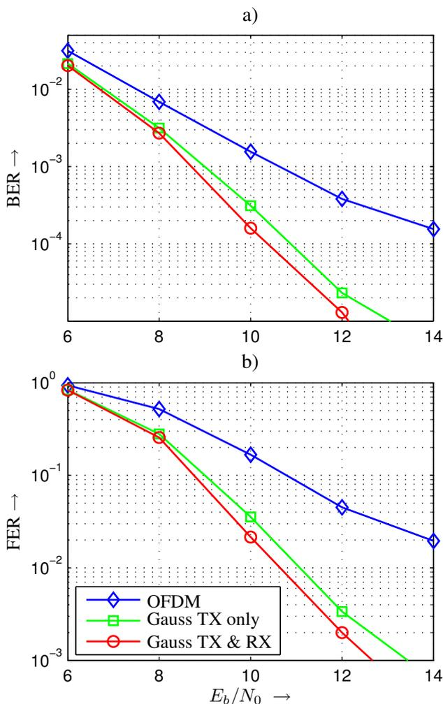
Fig. 4. Comparison of a) bit error rates and b) frame error rates for OFDM and the multicarrier system with truncated Gaussian impulses applied in the transmitter only as well as in the transmitter and receiver
