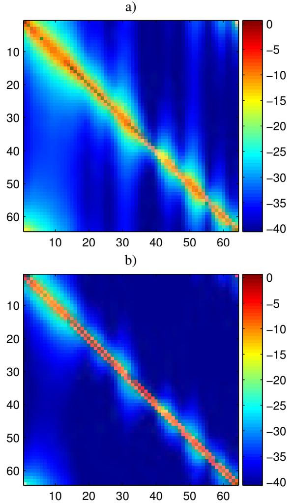
Fig. 2. Example of a  $(64 \times 64)$  channel matrix for a) OFDM and b) the multicarrier system with truncated Gaussian impulses ( $f_{3\text{dB}} T_s = 0.3$ ). The color shows the power of an element in dB.
