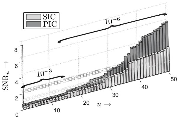
Fig. 6. SNR distributions for  $[5, 7]_o$  convolutional code and rate 1/10 repetition code, target BER=  $10^{-3}$  and  $10^{-6}$  respectively, 20 iterations
