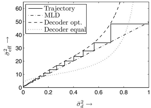
Fig. 7. Variance Transfer Chart for PIC with  $[5, 7]_o$  convolutional code and rate 1/10 repetition code, target BER  $10^{-3}$  and  $10^{-6}$  respectively,  $\bar{P} \cdot R_c / \sigma_n^2 \approx 15.7$  dB,  $\bar{P}$  is normalized to 1, 20 iterations
