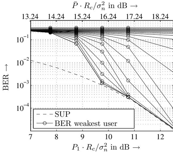
Fig. 9. Bit error rate of the weakest user for SIC using rate 1/20 repetition code
