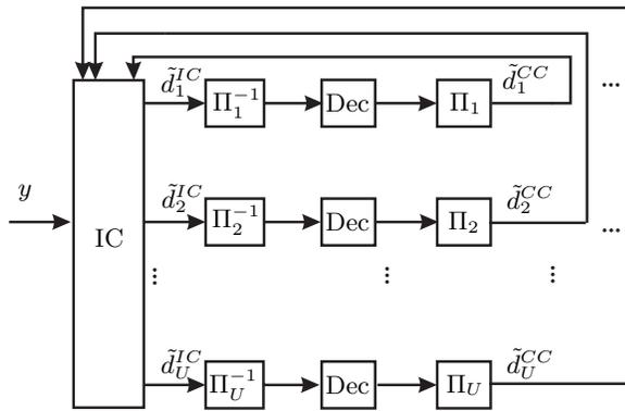
Fig. 2. Receiver structure of iterative parallel interference cancellation of an IDMA system
