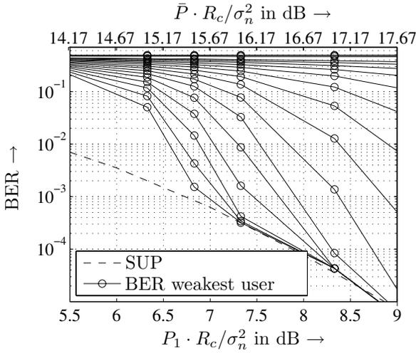
Fig. 10. Bit error rate of the weakest user for PIC using  $[5, 7]_o$  convolutional code and rate 1/10 repetition code
