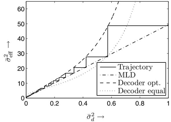
Fig. 3. Variance Transfer Chart for PIC, target BER  $10^{-3}$  and  $10^{-6}$  respectively,  $\bar{P} \cdot R_c / \sigma_n^2 \approx 17.6$  dB,  $\bar{P}$  is normalized to 1, 20 iterations
