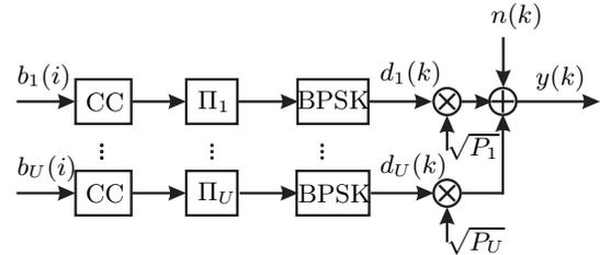
Fig. 1. Transmitter structure of an IDMA uplink system
