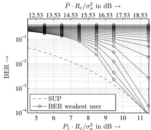
Fig. 8. Bit error rate of the weakest user for PIC using rate 1/20 repetition code
