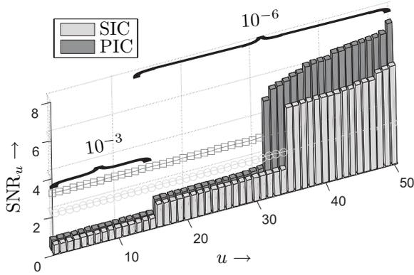
Fig. 5. SNR distributions for repetition code of rate 1/20, maximum BER=  $10^{-3}$  and  $10^{-6}$  respectively, 20 iterations
