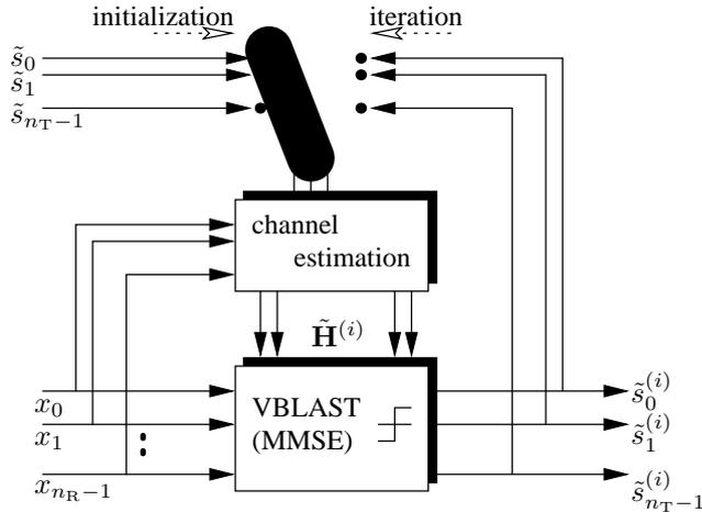
Fig. 5. improving the channel estimation / detection
