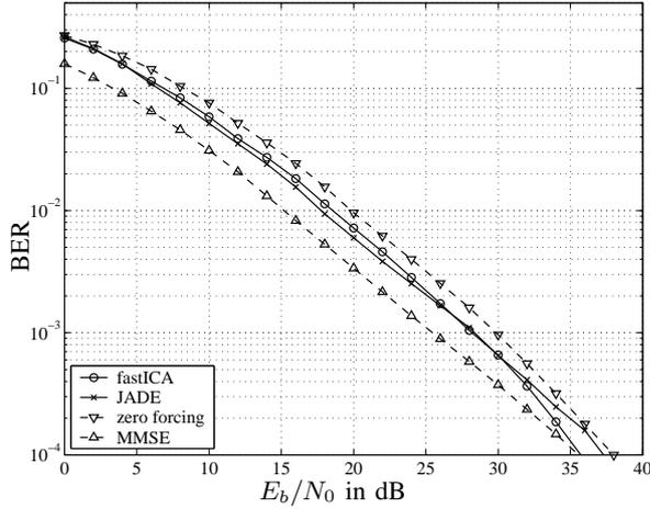
Fig. 4. BER error rates of the source separation approaches using HOS
