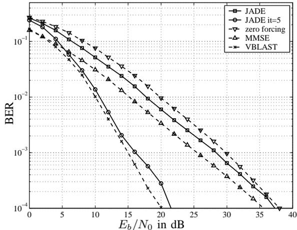
Fig. 6. BER of JADE with iterative VBLAST detection
