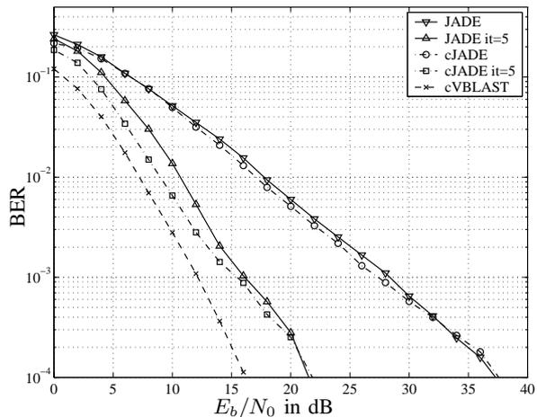
Fig. 8. BER of coded multi layer transmission
