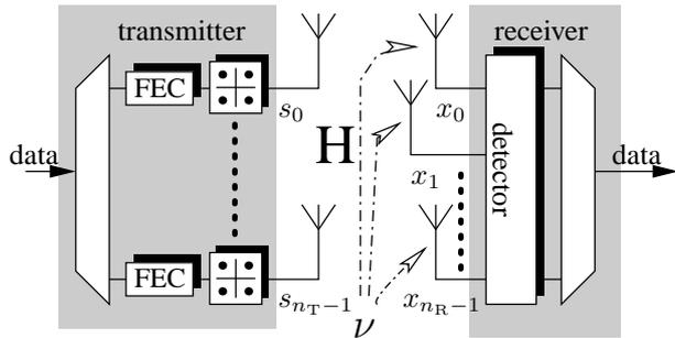
Fig. 7. transmission system with channel coding
