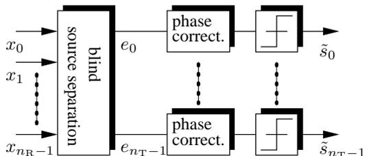
Fig. 2. source separation set up for BER measurements
