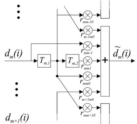
Fig. 2: Two-dimensional transmission model for MCSIS with  $r_{nmi} = r_{n,m}(iT)$
