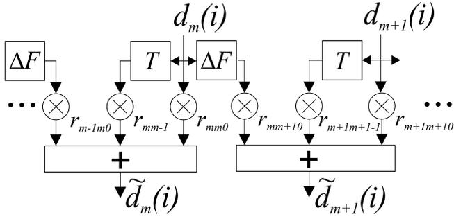
**Fig. 6:** Transmission model of the simple two-dimensional channel impulse response of Equation 7.
