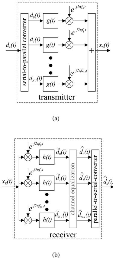
**Fig. 1:** Block diagram of a multicarrier system, (a): transmitter, (b): receiver
