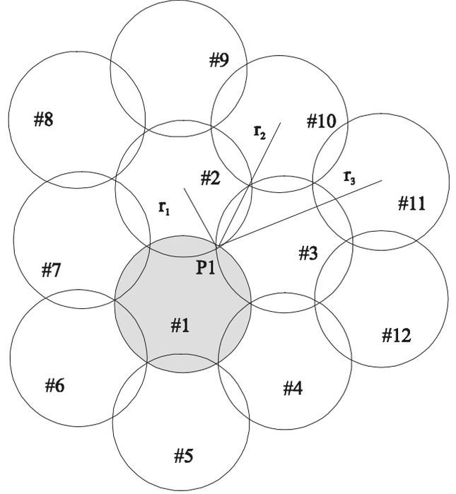
Fig. 2. Spot beam geometry
