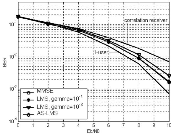
Fig. 5. Performance of the linear detector for long codes (worst case position, 10 users per spot beam, no coding, AWGN)
