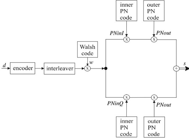
Fig. 1. Transmitter of the Globalstar system
