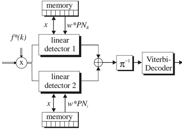
Fig. 4. Implementation of linear detectors for long codes
