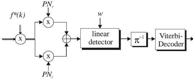
Fig. 7. Implementation of just one linear detector
