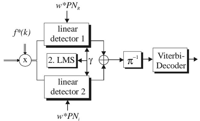
Fig. 6. AS-LMS detector with one second LMS-algorithm
