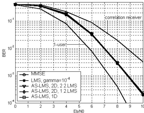
Fig. 8. Performance of the linear detector for long codes (worst case position, 30 users per spot beam, coding, Rice-channel)
