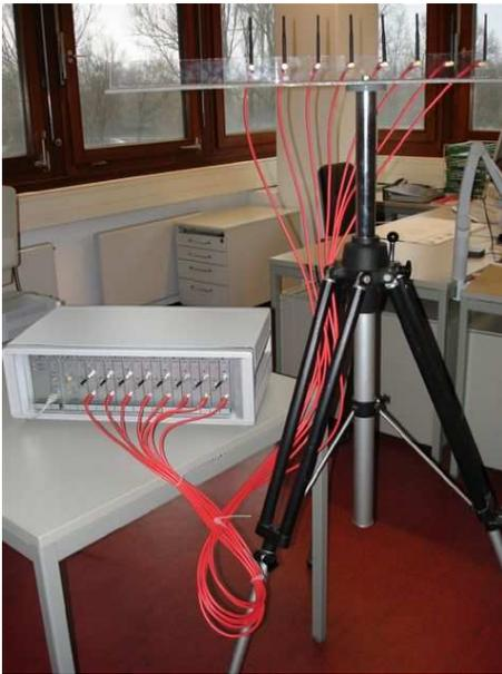
**Fig. 7:** The Multiple Antenna Transmitter for ISM-Band Transmission equipped with 8 modules.
