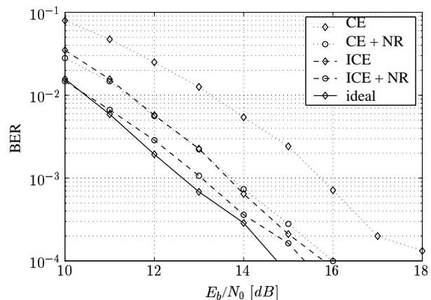
Fig. 2. Simulation results: BER *Hiperlan/2* conditions
