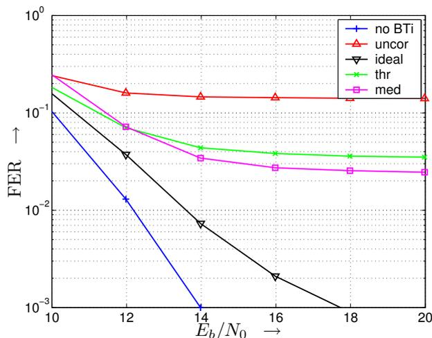
Fig. 7. Frame error rate of the 36 Mbit/s OFDM mode (16-QAM) in case of BT interference with SIR = 10 dB
