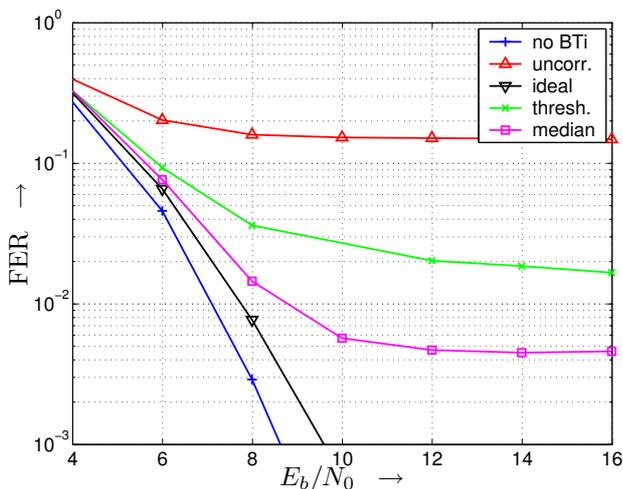
Fig. 6. Frame error rate of the 12 Mbit/s OFDM mode (QPSK) in case of BT interference with SIR = 0 dB
