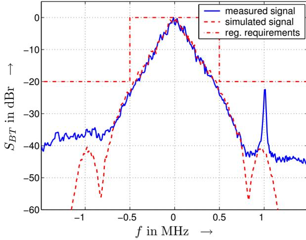
Fig. 2. Measured and simulated power density spectrum of a BT signal (one RF channel)
