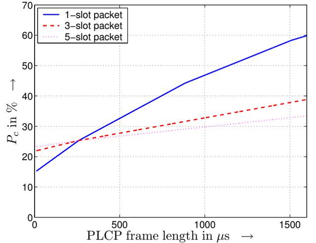
Fig. 1. Probability of collision with BT packet
