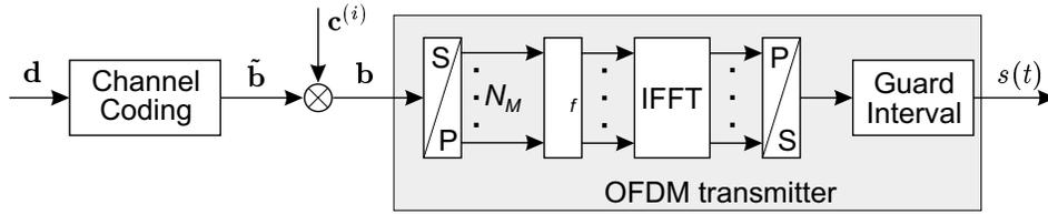
Fig. 1: Structure of coded OFDM-CDMA transmitter
