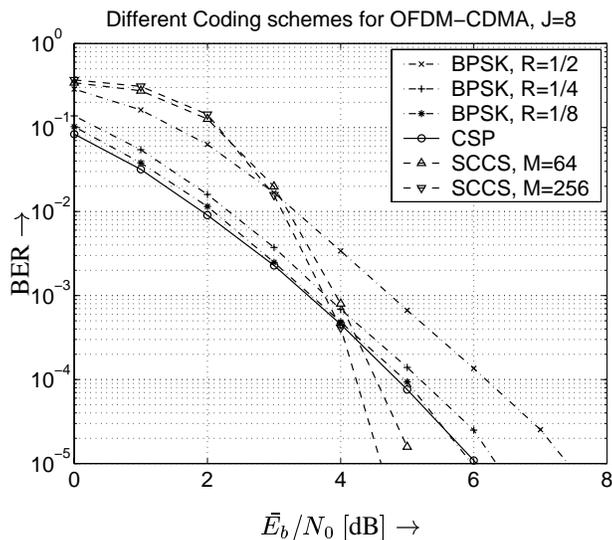
Fig. 7: Bit error rates for 4-path Rayleigh fading channel:  $J = 8$  user
