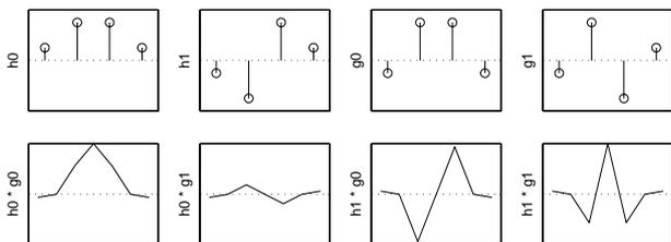
Fig. 2. The analysis and synthesis filters used in the example ( $h_0$ ,  $h_1$ ,  $g_0$  and  $g_1$ ) and their pair-wise convolutions.
