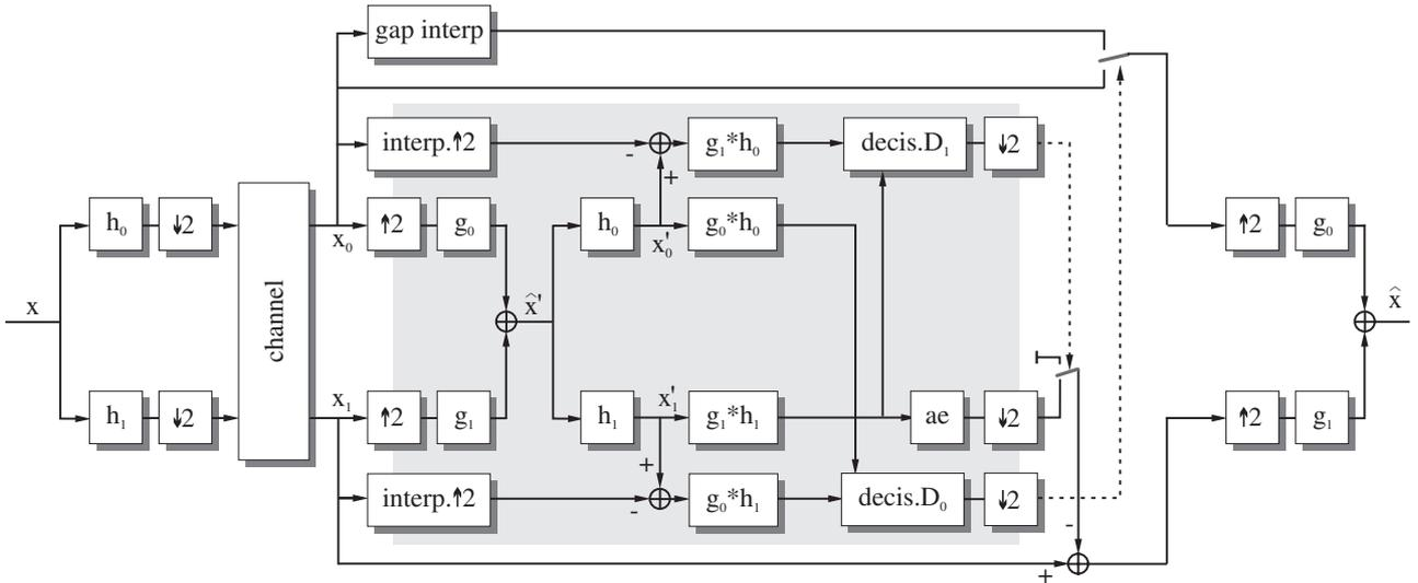
Fig. 3. The 1D subband analysis and error correcting synthesis.
