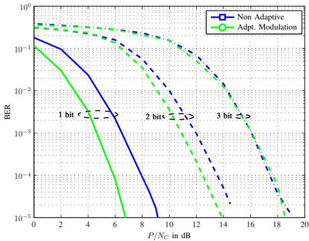
Fig. 6. BER vs. transmit power  $P$ , frequency selective channel with  $L = 10$  equal power taps,  $N_C = 64$  subcarriers, modulation 16-QAM, Turbo code ( $R_C = 1/2$ , 8 decoder iterations) over one OFDM symbol
