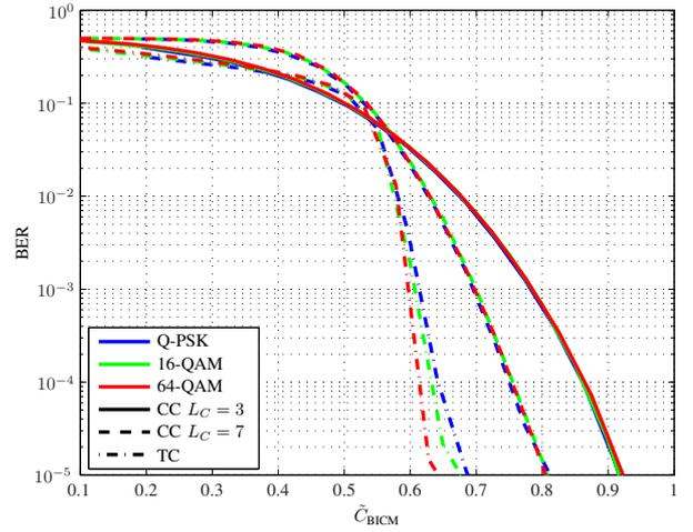
Fig. 2. Comparison of the BER vs.  $C_{\text{BICM}}$  with regard to two convolutional codes ( $R_C = 0.5$  with  $L_C = 3$  (solid),  $L_C = 7$  (dashed)) and one turbo code (dash dotted) applying Q-PSK (blue), 16-QAM (green) and 64-QAM (red);  $N_C = 1024$  subcarriers,  $L_F = 10$  channel taps
