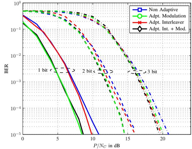
Fig. 5. BER vs. transmit power  $P$ , frequency selective channel with  $L = 10$  equal power taps,  $N_C = 1024$  subcarriers,  $[171, 133]_8$  convolutional code ( $R_C = 1/2$ ,  $L_C = 7$ ) over one OFDM symbol; QPSK (solid), 16-QAM (dashed), 64-QAM (dash dotted)
