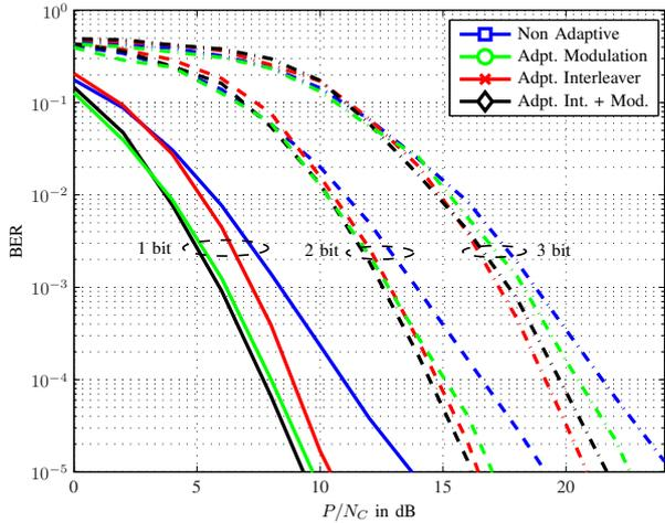
Fig. 4. BER vs. transmit power  $P$ , frequency selective channel with  $L = 10$  equal power taps,  $N_C = 1024$  subcarriers,  $[7, 5]_8$  convolutional code ( $R_C = 1/2$ ,  $L_C = 3$ ) over one OFDM symbol; QPSK (solid), 16-QAM (dashed), 64-QAM (dash dotted)
