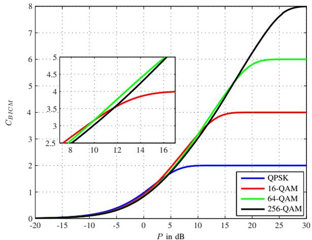
Fig. 3. Bit Interleaved Coded Modulation capacity for the modulation schemes QPSK, 16-QAM, 64-QAM and 256-QAM using binary reflected gray-mapping for an AWGN channel with noise power  $\sigma_n^2 = 1$  and power  $P$
