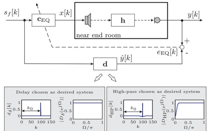
**Figure 1:** Least-squares equalizer  $\mathbf{c}_{\text{EQ}}$  for listening-room compensation and two possible desired systems  $d_\delta[k]$  (delay) and  $d_{\text{HP}}[k]$  (delayed high-pass) in time and frequency domain.
