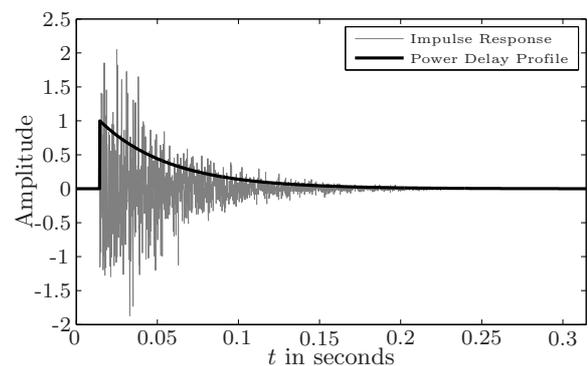
**Figure 4:** RIR and power delay profile (PDP).
