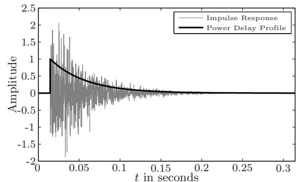
**Figure 4:** RIR and power delay profile (PDP).
