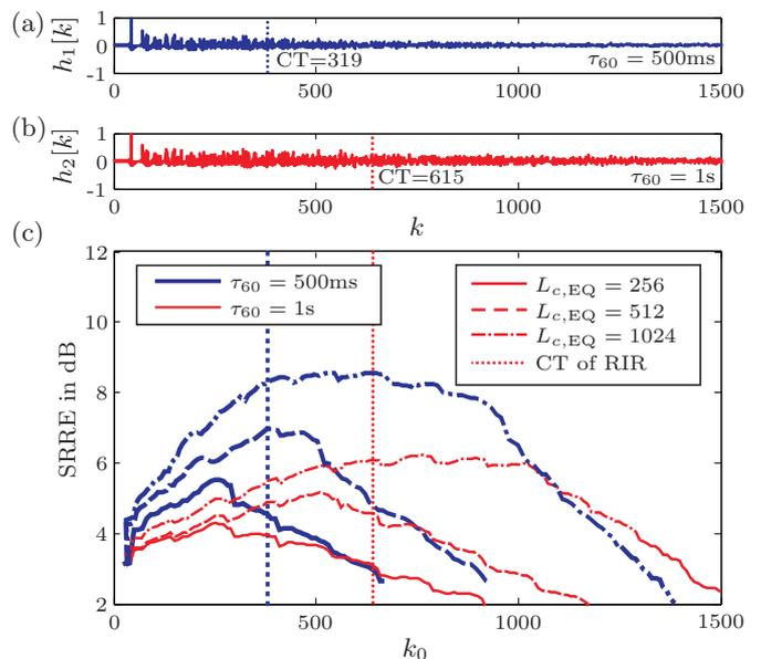
**Figure 2:** (a) RIR with reverberation times of  $\tau_{60} = 500\text{ms}$  and its CT in samples. (b) RIR with  $\tau_{60} = 1\text{s}$  and its CT. (c) equalizer performance in dependence of delay  $k_0$  of the desired system for different equalizer filter lengths  $L_{c,EQ}$  and RIRs (a) (thicker blue lines) and (b) (thinner red lines).
