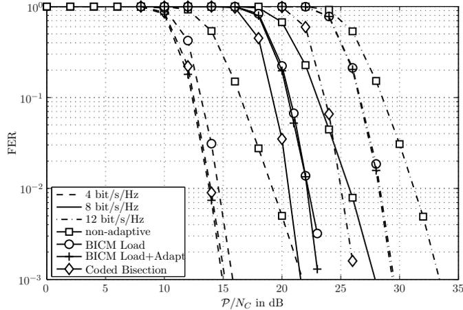
Figure 3. FER vs average power per subcarrier  $\mathcal{P}/N_C$  for ZF receive filtering and convolutional codes of constraint length  $L_C = 3$ ;  $N_C = 1024$  subcarriers,  $N_T = N_R = 4$  antennas,  $L_F = 10$  channel taps
