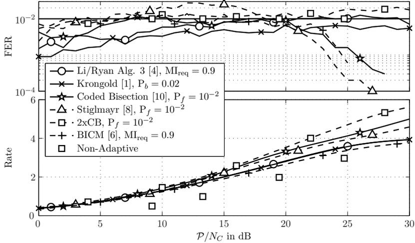
Figure 1. FER and Rate vs average power per subcarrier  $P/N_C$  for convolutional codes of constraint length  $L_C = 3$ ;  $N_C = 1024$  subcarriers,  $L_F = 10$  channel taps, target FER of  $P_{\text{Target}} = 10^{-2}$
