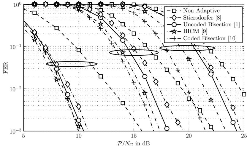
Figure 2. FER vs average power per subcarrier  $\mathcal{P}/N_C$  for convolutional codes of constraint length  $L_C = 3$  at spectral efficiencies of 1, 2 and 3 bit/s/Hz (left to right);  $N_C = 1024$  subcarriers,  $L_F = 10$  channel taps
